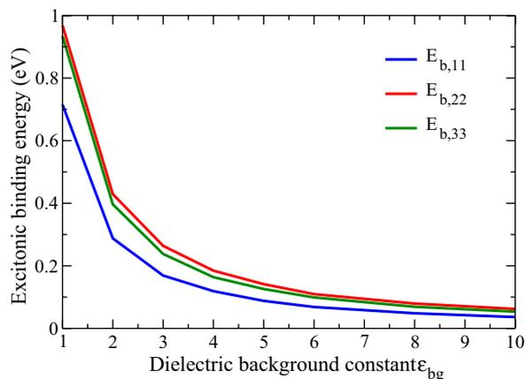
**Figure 2** (online color at: [www.pss-b.com](http://www.pss-b.com)) Excitonic binding energies for the first three transitions of the exemplary (10,0) zigzag nanotube are plotted as a function of the dielectric background constant  $\epsilon_{bg}$ . The figure illustrates the influence of the surrounding medium on excitonic properties of carbon nanotubes.
