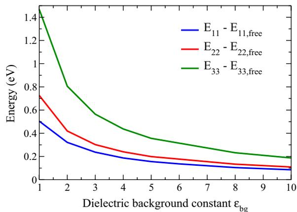
**Figure 3** (online color at: [www.pss-b.com](http://www.pss-b.com)) The excitation energies of the first three transitions of the exemplary (10,0) zigzag nanotube are plotted as a function of the dielectric background constant  $\epsilon_{bg}$ . For reasons of a better comparison between different transitions, we shifted the excitation energies by the value of the corresponding free particle energies with  $E_{11,free} = 1.00$  eV,  $E_{22,free} = 2.18$  eV, and  $E_{33,free} = 3.52$  eV.
