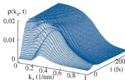
**Figure 4** (online color at: [www.pss-b.com](http://www.pss-b.com)) Carrier dynamics in the exemplary (11,6) semiconducting nanotube after excitation above the excitonic resonance.
