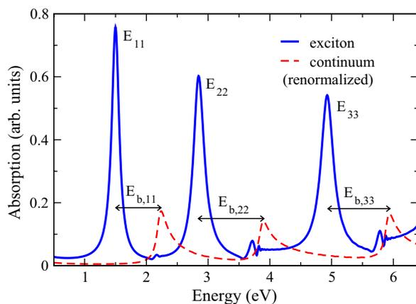
**Figure 1** (online color at: [www.pss-b.com](http://www.pss-b.com)) Optical absorption spectrum of the (10,0) zigzag nanotube. The energetically lowest three transitions are shown. The blue solid line illustrates the spectrum containing excitonic effects, while the dashed red line shows the free particle spectrum, which already includes the renormalization due to the electron–electron coupling. The arrows indicate the corresponding excitonic binding energies.
