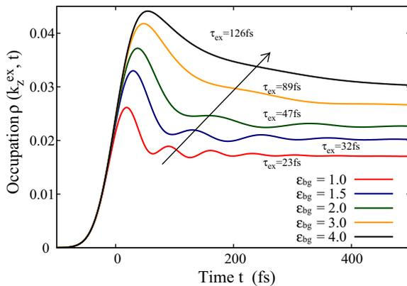
**Figure 5** (online color at: [www.pss-b.com](http://www.pss-b.com)) Carrier relaxation in the exemplary (11, 6) semiconducting nanotube for different dielectric background constants  $\epsilon_{bg}$ . The higher  $\epsilon_{bg}$ , i.e., the larger the external screening, the slower is the relaxation dynamics and the less pronounced are the plasma oscillations.
