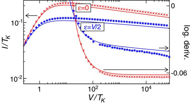
Fig. 2: (Color online)  $I(V)$  for the symmetric model with  $U_L = U_R = 0.1/\pi$  obtained from the numerical solution of the full RTRG-FS (lines) and FRG (symbols) equations; crosses:  $\epsilon = 0$ ; stars:  $\epsilon = V/2$ .
