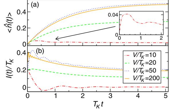
Fig. 5: (Color online) Time evolution of the dot occupation  $\langle \hat{n}(t) \rangle$  and the current  $I(t)$  for  $U_L = U_R = 0.1/\pi$ ,  $\epsilon = 10 T_K$ , and the initial condition  $\langle \hat{n}(0) \rangle = 0$  (see footnote <sup>4</sup>). At times  $t \lesssim 2/T_K$  we observe an oscillating behavior.
