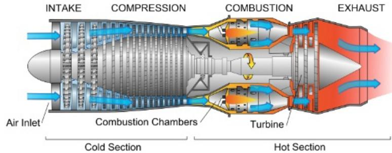
Figure 1: Cross section of a jet engine
