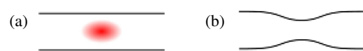
FIG. 1. Examples of impurities in twisted bilayer graphene (schematically shown as black lines), which are (a) even (charged impurity located between the layers; schematically shown in red) and (b) odd (local change in interlayer tunneling) under \mathcal{PT} ( \mathcal{P} and \mathcal{T} denote particle-hole and time-reversal conjugation, respectively). \mathcal{PT} -even impurities induce subgap states in the K-IVC phase of TBG, while \mathcal{PT} -odd impurities do not due to Anderson's theorem for the K-IVC state.
