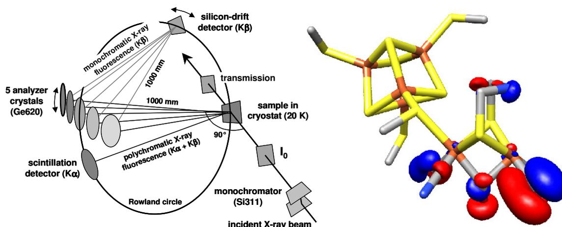
Setup for high-resolution XAS/XES at ESRF (left) and molecular orbitals from DFT calculations on the H-cluster of [FeFe] hydrogenase (right).
