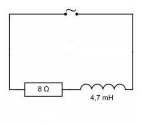
Fig. 8: RL Circuit for use as a low-pass filter. The measuring instruments and connections for the output voltage are not shown.
