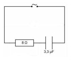
Fig. 7 RC circuit for use as a high pass filter. The measuring instruments and the connections for the output voltage are not shown.
