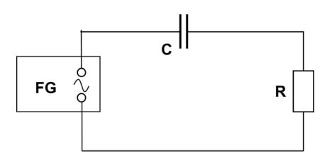
Fig. 6: R-C circuit for recording the charge and discharge curves of a capacitor of capacitance C. The function generator FG serves as voltage source. The resistor R is required for current limitation. The oscilloscope for observing the charge and discharge curve is not shown.
