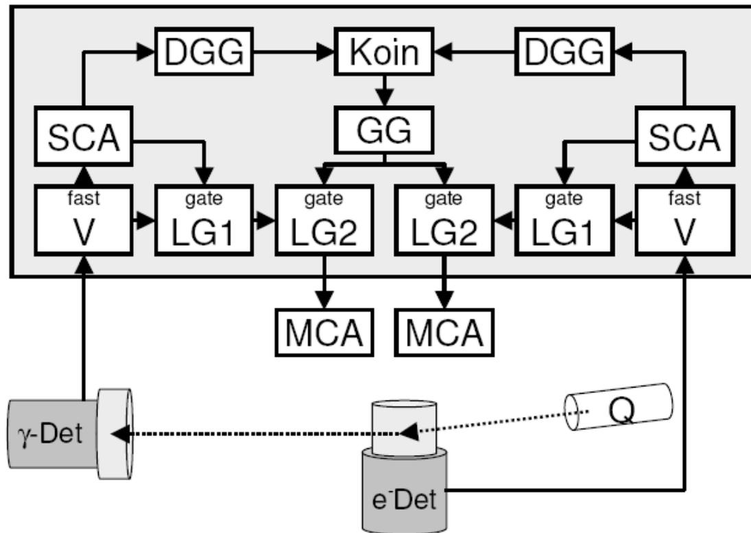
Figure 1: The block diagram is shown in the upper part of the picture (for explanation of abbreviations see equipment list). Note that the actual detector signal from the amplifier V via the linear gates (LGs) to the MCA pass depending on whether the control inputs (gates) of the LGs are enabled or not. The detection of the coincidence and blocking of random coincidences is done by the other components.
