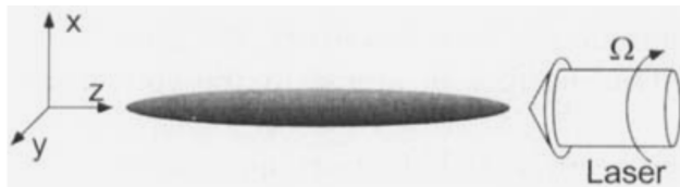
Figure 1 – A cigar-shaped condensate is confined by an axisymmetric magnetic trap and stirred by an off-center far-detuned laser beam. The laser beam propagates along the long axis and creates an anisotropic quadrupole potential that rotates at an angular velocity \Omega . The image is taken from Ref. [14].
