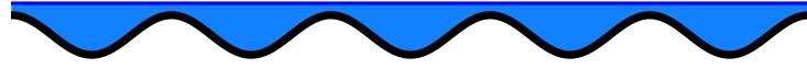
Figure 1.8 – Superfluid ground state. Particles are delocalized (blue region) through the whole lattice volume (black line).
