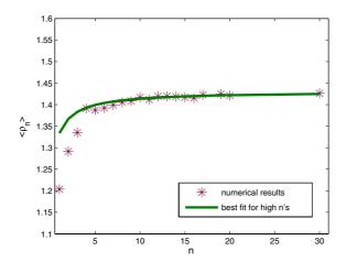
**Figure 5.** The measured value of  $\langle \rho_n \rangle$  compared to the best numerical fitting (for high values of n) to (17):  $\langle \rho_n \rangle = \sqrt{2}(n + 0.805)/(n + 0.936)$ .
