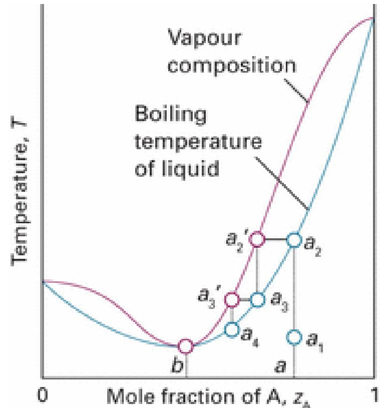
A low-boiling azeotrope. When the mixture at  $a$  is fractionally distilled, the vapour in equilibrium in the fractionating column moves towards  $b$  and then remains unchanged.
