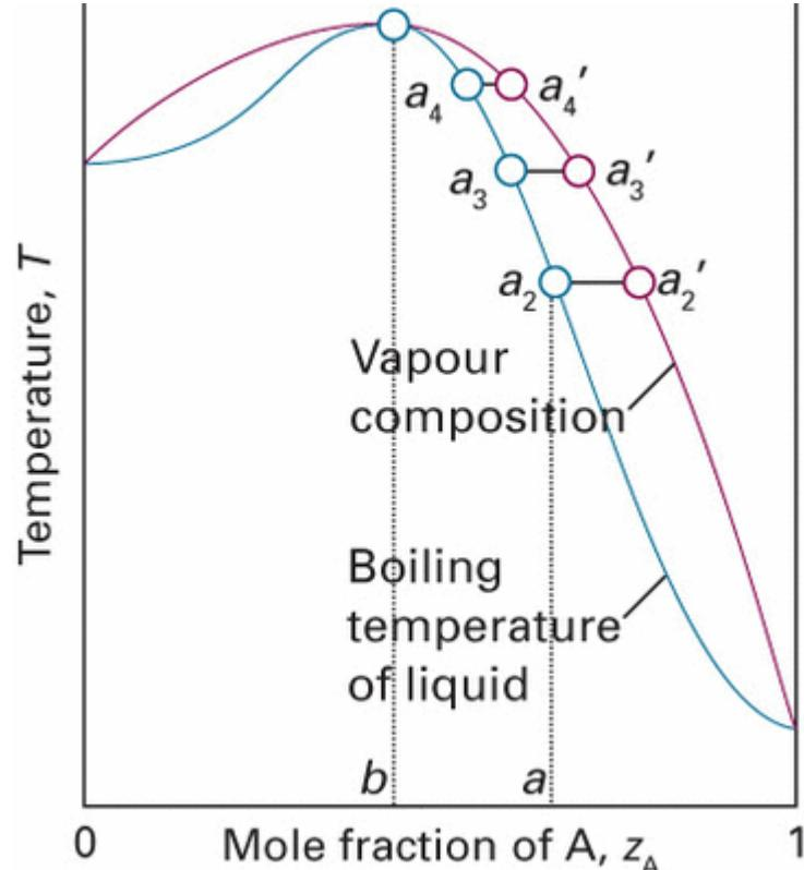
A high-boiling azeotrope. When the liquid of composition  $a$  is distilled, the composition of the remaining liquid changes towards  $b$  but no further.
