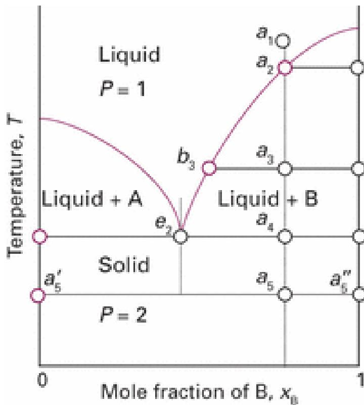
The temperature–composition phase diagram for two almost immiscible solids and their completely miscible liquids
