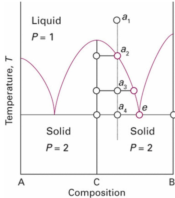
The phase diagram for a system in which A and B react to form a compound C = AB
