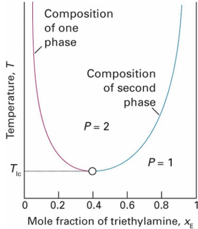
The temperature–composition diagram for water and triethylamine. This system shows a lower critical temperature at 292 K. The labels indicate the interpretation of the boundaries.
