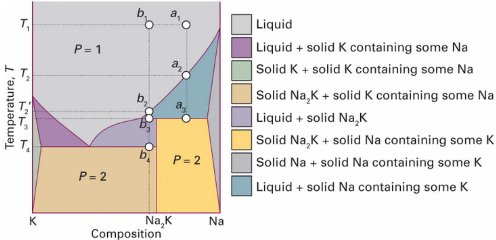
The phase diagram for an actual system (sodium and potassium).
