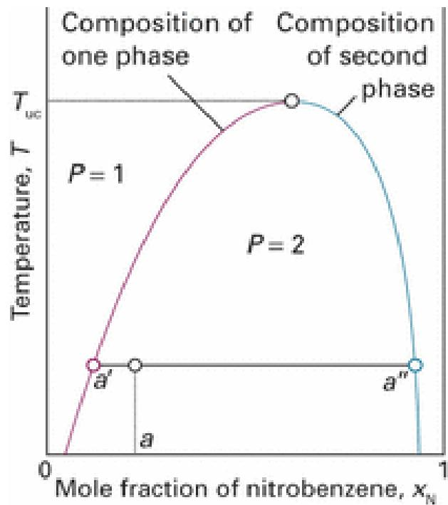
The temperature–composition diagram for hexane and nitrobenzene at 1 atm. The region below the curve corresponds to the compositions and temperatures at which the liquids are partially miscible. The upper critical temperature,  $T_{uc}$ , is the temperature above which the two liquids are miscible in all proportions.
