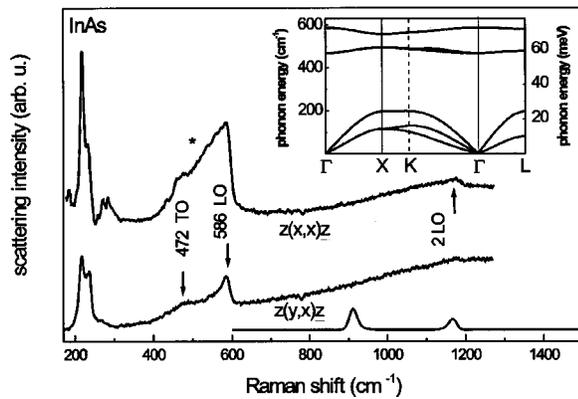
FIG. 3. First-order and second-order Raman spectra of cubic InN taken at room temperature for  $z(x,x)\bar{z}$  and  $z(y,x)\bar{z}$  configurations. The excitation wavelength was 632.8 nm, in resonance with the band gap of InN. The high intensity marked by \* is caused by the second-order signal of InAs. The lowest curve shows the calculated density of states of the overtones. In the inset we present the calculated phonon dispersion curves of cubic InN.
