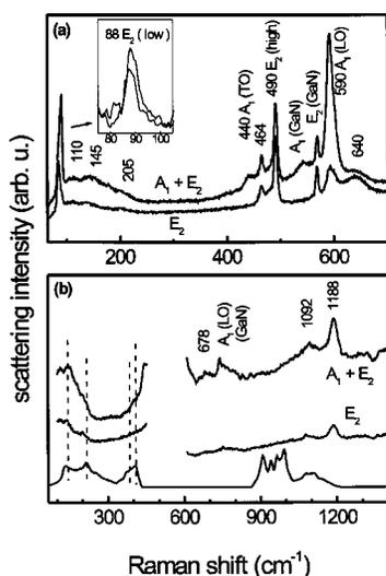
FIG. 1. First-order (a) and second-order (b) Raman spectra of hexagonal InN taken at room temperature for scattering geometries corresponding to  $A_1+E_2$  and  $E_2$  symmetries. The lowest trace in (b) shows the calculated density of states. The excitation wavelength was  $632.8$  nm (first order) and  $488$  nm (second order). The inset ( $\lambda_{\text{exc}}=488$  nm) shows the  $E_2$  (low) mode for both scattering configurations.
