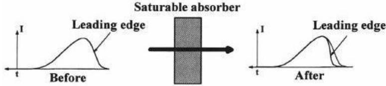
Figure 2: Schematical representation of the operation of a saturable absorber [2]. The leading edge of the incoming pulse is diminished while the peak is not, as the SA is already saturated. For slow SA, the trailing edge won't be absorbed since the relaxation time is longer than the peak duration.
