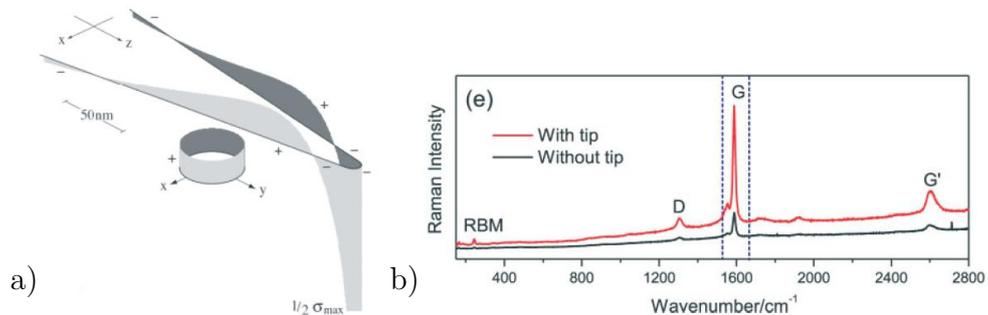
Figure 6: a) Simulation of the charge density depending on the position at the surface of the tip. A large electron concentration at the tip apex is visible. The graph is rotationally symmetric. b) Measured Raman spectrum with (red) and without (black) TERS. The whole spectrum is enhanced due to localized SPPs in the tip. [7]
