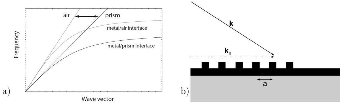
Figure 4: a) Dispersion relation of light and SPP in different media. The dispersion relations for the same propagation medium only cross at  $k = 0$  forbids excitation of SPPs. At an interface of metal, air and prism coupling is allowed. b) Excitation of SPPs are also possible using gratings, where a phase matching condition imposes restrictions upon the wave vector of the incoming light. [5]
