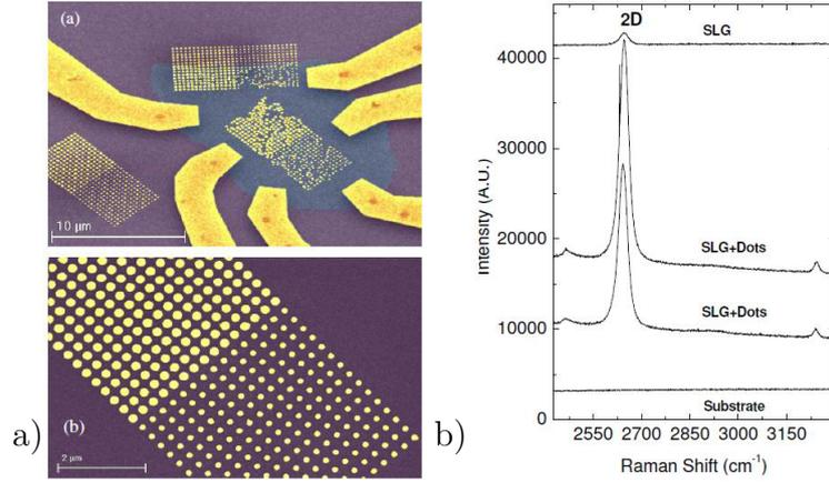
Figure 5: a) Arrangement of NPs (yellow) on SiO (purple) and a SLG sample (blue). b) Raman signal in the vicinity of the 2D peak. A huge enhancement of the signal with NPs compared to normal graphene can be seen. [6]
