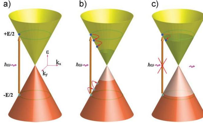
Figure 3: Excitation and saturation process at the K-point of the graphene bandstructure [3]. a) Incoming light creates excited electrons in the conduction band. b) Electrons relax within the conduction band due to pair-carrier and electron-phonon collisions and thus fill up all available states from the bottom of this band. c) All possible states for excitations are filled so further incoming light cannot cause transitions anymore (Pauli blocking), the SA is saturated.
