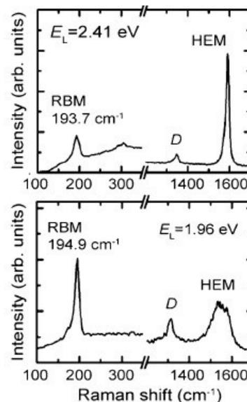
**Fig. 11: Broadening of the high-energy peak in metallic tubes. Ref. [9]**
