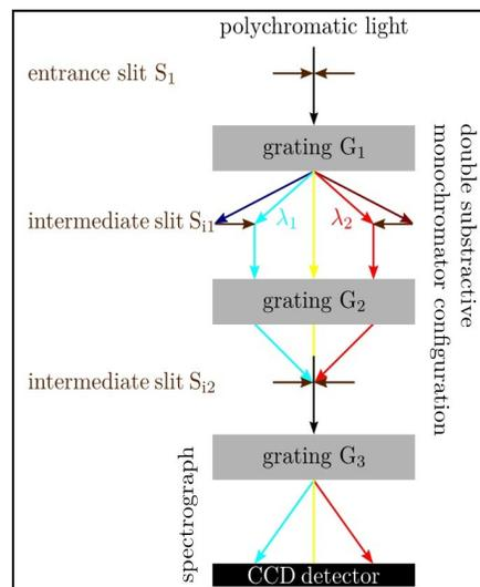
**Fig. 7: Triple monochromator used to remove the Rayleigh light from the signal. Ref. [5]**
