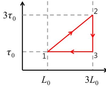
Fig. 2: The heat engine cycle of a rubber band.
