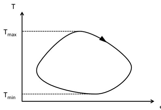
Figure 1: Example of an arbitrarily shaped cyclic process in a  $T - S$  diagram.
