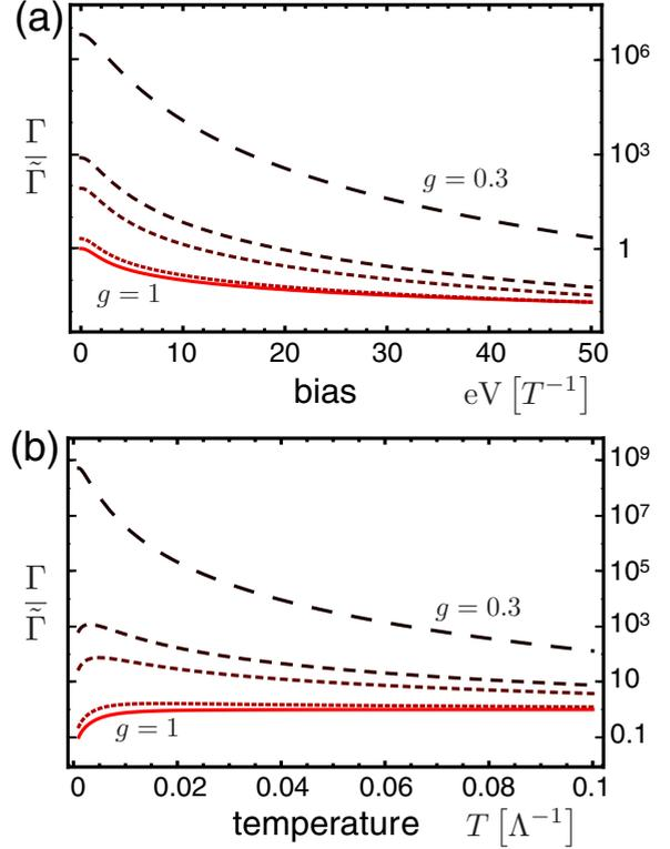
FIG. 3. Log-plot of the ratio between local-density-induced and tunneling-induced decoherence as a function of (a) bias voltage and (b) temperature; cf. Eqs. (12) and (15). For increasing interaction strength  $g = 1, 0.9, 0.6, 0.5, 0.3$  from light to dark red and from continuous to coarsely dashed.  $\frac{T}{\Lambda_g} = 0.01$  in (a) and  $\frac{eV}{\Lambda_g} = 0.01$  in (b),  $\tilde{\lambda}_2 - \tilde{\lambda}_1 = \lambda_2 - \lambda_1 = \Delta\lambda$ .
