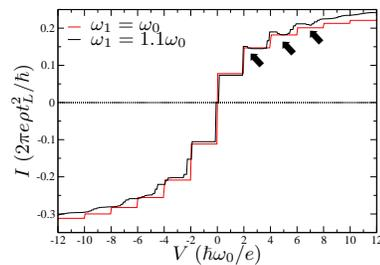
FIG. 2: (Color online) Current-voltage characteristics for an asymmetric device ( $t_R^2 = 0.3t_L^2$ , symmetric voltage splitting) in the unequilibrated regime with  $\lambda = 1.1$ ,  $k_B T \ll \hbar\omega$ ,  $U \rightarrow \infty$ . The combination of asymmetric coupling and differing vibrational frequencies is observed to lead to weak peaklike structures at the onsets of phonon steps with negative differential conductance regions (marked by arrows).
