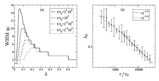
FIG. 3. (a) Width of the phonon distribution as a function of electron-phonon coupling strength for several vibrational relaxation times  $\tau$  and  $eV=3\hbar\omega$ ,  $k_BT=0.05\hbar\omega$ ,  $\epsilon=0$ . For  $\lambda>0.25$  all curves show the approximate  $q_0\sim\lambda^{-1}$  scaling. Below a relaxation-rate-dependent crossover point  $\lambda_0$ , the WHM is strongly suppressed due to direct relaxation. (b) Crossover point  $\lambda_0$  vs relaxation time  $\tau$ .
