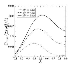
FIG. 4. Mean dissociation rate as a function of electron-phonon coupling strength at  $k_BT$ =0.005 $\hbar\omega$  for several bias voltages as obtained by Monte Carlo simulation with a Morse potential containing ten bound states.
