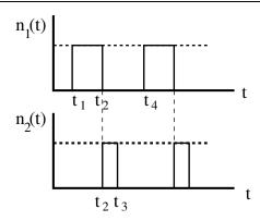
FIG. 2. Schematic time evolution of occupations  $n_1(t)$  and  $n_2(t)$  of levels 1 and 2, respectively, in the active layer under conditions of a finite current.
