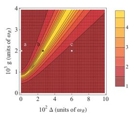
FIG. 2. (Color online) Fano factor for different values of detuning and coupling between qubit and resonator. Points a, b, and c are defined as in Fig. 1.
