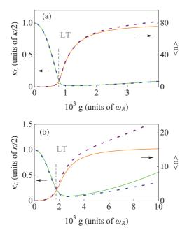
FIG. 6. (Color online) Average photon number and linewidth as functions of the coupling strength on resonance with (a)  $\kappa=10^{-4}\omega_R$  and (b)  $\kappa=5\times10^{-4}\omega_R$ . Results obtained from the DILE and the FPE methods are represented by the solid and the dashed lines, respectively.
