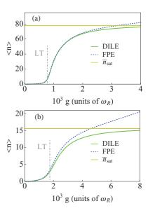
FIG. 3. (Color online) Average photon number on resonance obtained from the DILE (solid) and the FPE approach (dotted). Parameters are (a)  $\kappa = 10^{-4}\omega_R$  and (b)  $\kappa = 5 \times 10^{-4}\omega_R$ . The dot-dashed line indicates the lasing threshold (LT) estimated using Eq. (14).
