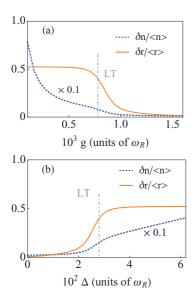
FIG. 4. (Color online) (a) Relative fluctuations as function of g at resonance and (b) as function of  $\Delta$  at  $g=0.002\,\omega_R$ . In both panels  $\kappa=10^{-4}\omega_R$ .
