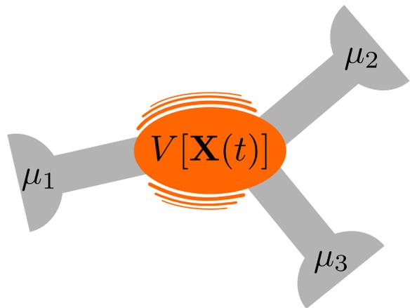
FIG. 1: Example of a scattering system that is coupled to slow classical degrees of freedom  $\mathbf{X}(t)$ . The movement of the scatterer changes the scattering potential  $V[\mathbf{X}(t)]$ . The backaction of the electrons passing through the scatterer then leads to reaction forces acting on  $\mathbf{X}(t)$ .
