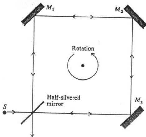
Figure I.6. Diagram of Sagnac's experiment.
