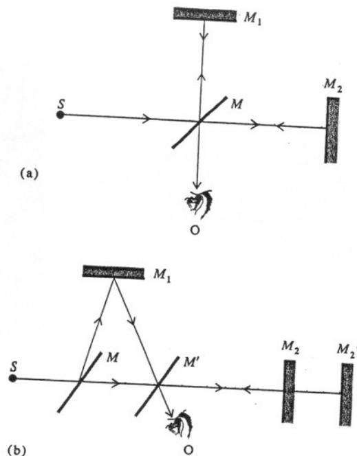
Figure I.1. Simplified diagram of the Michelson-Morley experiment.
