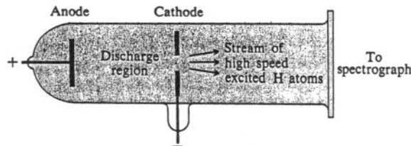
Figure I.4. Discharge tube used to observe the relativistic Doppler effect.
