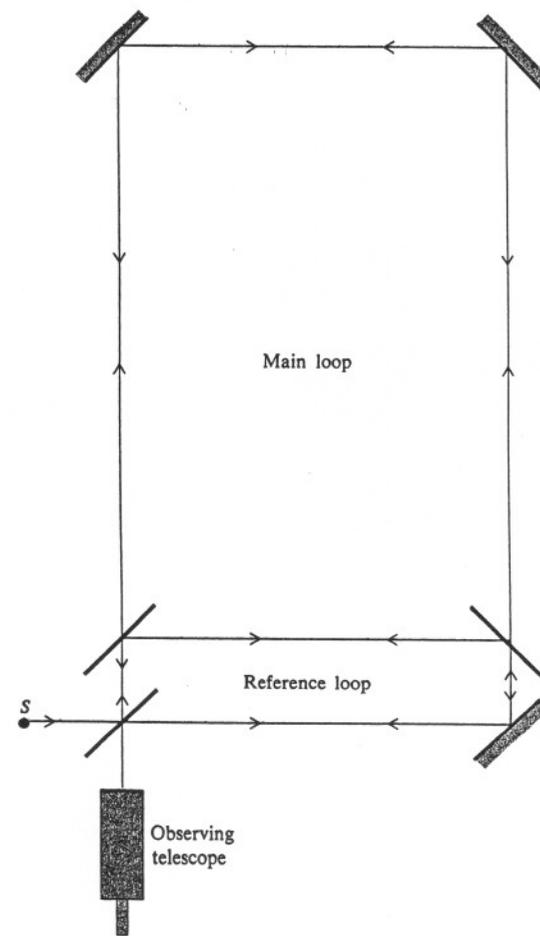
Figure I.7. The Michelson-Gale experiment for detecting the absolute rotation of the earth.
