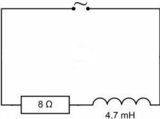
Fig. 8: RL Circuit for use as a low-pass filter. The measuring instruments and connections for the output voltage are not shown.
