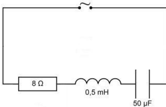
Fig. 9: RLC Circuit for use as a band-pass filter. The measuring instruments and the connections for the output voltage are not shown.
