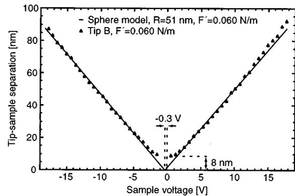
FIG. 3. The curve indicated by triangles shows how the tip-to-sample separation  $d$  varies with sample voltage  $U$  at a constant force gradient of 0.060 N/m, using the B tip. The solid curve represents  $d(U+0.3\text{ V})$  using the analytical expression for the sphere model describing the electrostatic interaction. The 0.3 V offset is due to the contact potential.
