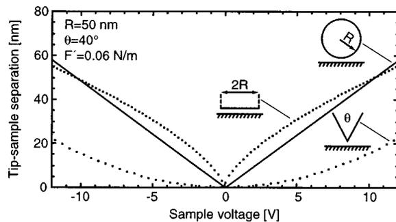
FIG. 2. Theoretical curves showing how the tip-to-sample distance varies with sample voltage if the force gradient is kept constant. The three curves correspond to the electrostatic interaction models presented in Table I. Tip and sample are presumed to be metallic, and the tip is held at ground potential. The parameters are chosen to match the experimental values for tip B used in Fig. 3.
